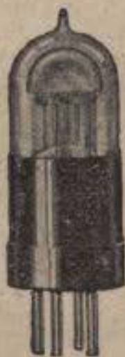
The Wuncell Dull Emitter Voltage 178 volts. Consumption 3 amp. W 1 for Detector and I. F. 14/- W 2 for H. F. amplification 14/- W 3 Cossor Loud Speaker Valve Voltage 178 volts. Consumption 3 amp. Price 18/6
